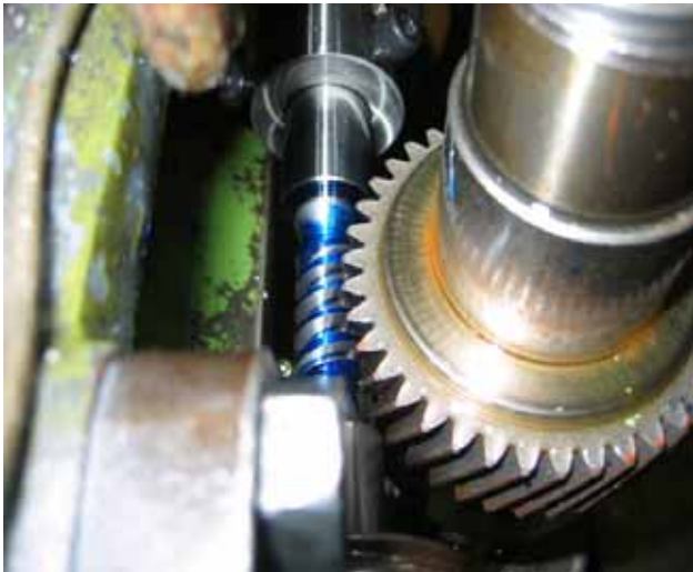
Fig.7 Grinding of Modifying Hindley Worm by the Involute helical gear grinder, on which the diamond abrasive grains are attached
