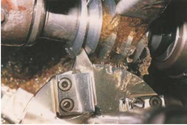
Fig. 6 Cutting of Modifying Hindley Worm by Pinion Cutter with straight lined tool
