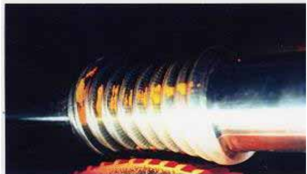
Fig.5 Modifying Hindley Worm Gear ground by cone shaped grinder
