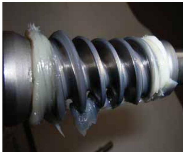
Fig.20 Tooth Contact Mark of Worm teeth after Running test
