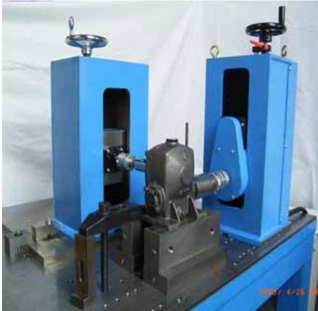
Fig.22 M-MATE calculating the angular transmission error
