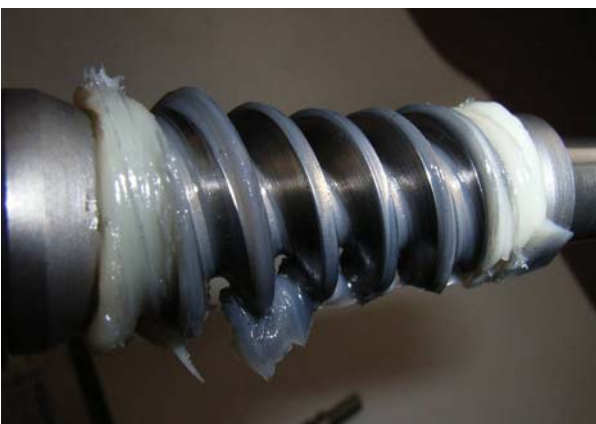
Fig.5 Tooth contact mark on the worm tooth after experiment.
