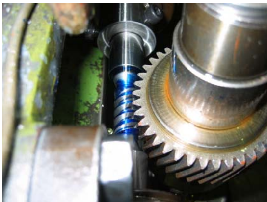
Fig.8 Grinding of the worm teeth by the involutes helical gear shaped grinder
