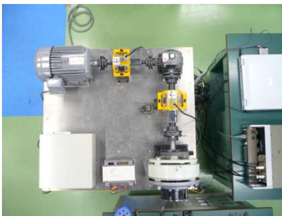
Fig.11 Worm gear testing machine of power absorption type. The authors designed and made the worm gear
