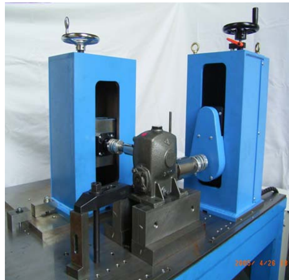
Fig. 9 Photo of M-MATE (abbreviated from M easuring- M achine for the A ngular T ransmission E rror of the Reducer)
