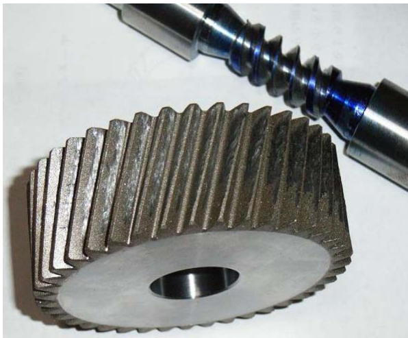
Fig.7 The involutes helical gear shaped grinder on which the diamond abrasive grains are attached and the finished worm.
