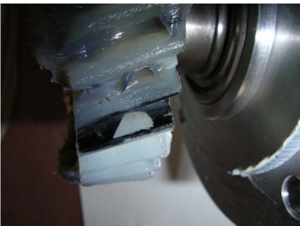
Fig. 4 Tooth contact mark on the wheel after experiment.
