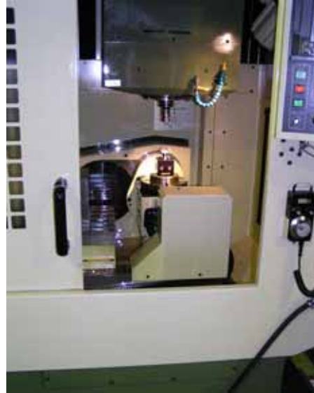
Fig. 7 Manufacturing master gears for electrode by machining center using ball endmil.
