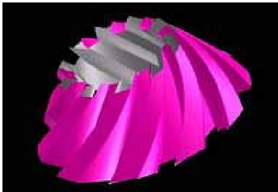
Fig. 6 3D expression of electrode of pinion drawn by 3D /CAD software.
