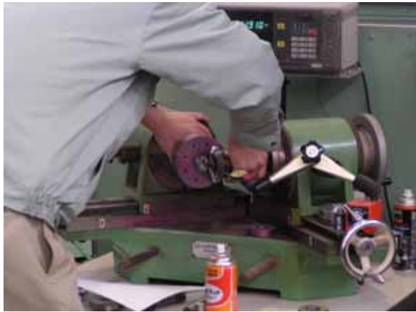
Fig.10 Testing the tooth contact of the master pinion and gear.
