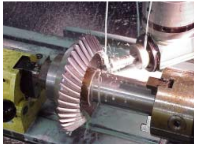
Fig.9 Processing of WN spiral bevel gear by marching center
