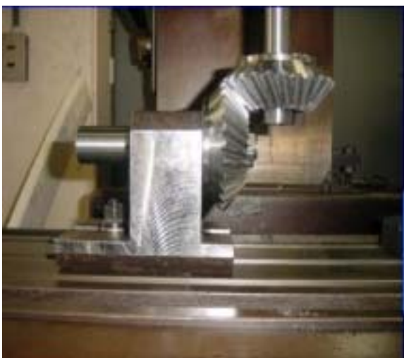
Fig.12 Apparatus for experiment of TCA applying Milling machine
