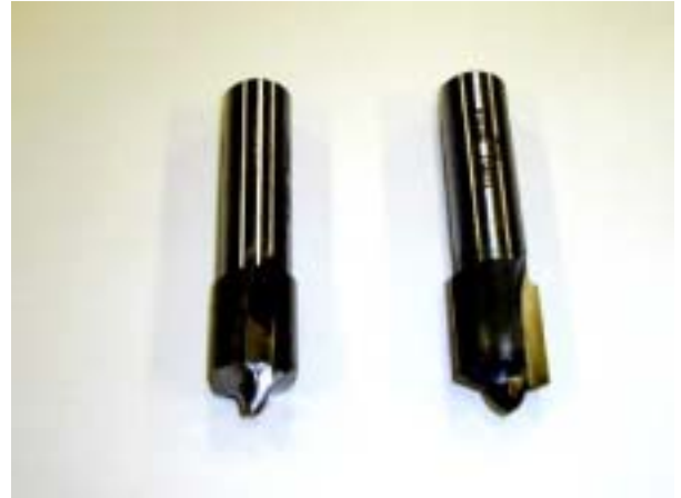
Fig.8 Completed volcanic shape end mill and spherical end mill
